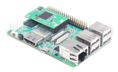
Geniatech's XPI-3288 is a cost-effective open source motherboard, powered by The Rockchip RK3288 quad-core Cortex-A17, with a main frequency up to 1.8 GHZ, stable operation, strong hard decoding capability and rich expansion interfaces.
