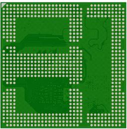
The SoM-IMX8MM-OSM core board is an embedded System on Module developed according to the latest OSM (Open Standard Modules™) standard released by SGeT (Standardization Group for Embedded Technology eV). It adopts NXP's iMX-8M-Mini processor with 2GB LPDDR4 and 8GB eMMC storage.
