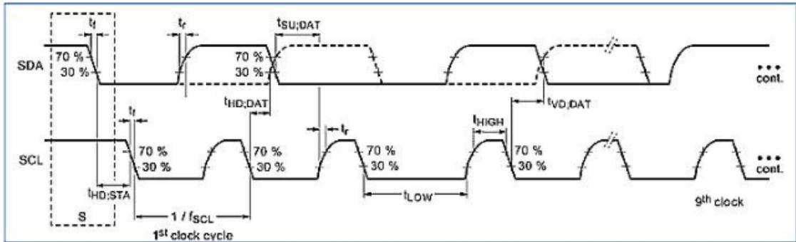
8.2.3 If the above two items are not configured, the calculation will be based on the max value of the rising edge and the falling edge by default, and the clk speed obtained will be nearly 90k. The default max value of 100k is 1000ns, which is in line with most hardware, so if the requirement is not high, it can not be configured.
