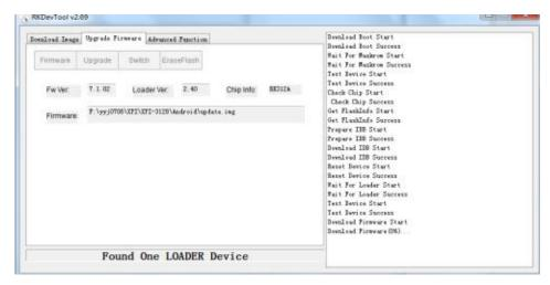
1 ) Click the firmware to select the newly packaged update.img file, and click the upgrade button to download. (Note that the device must be in download mode).
