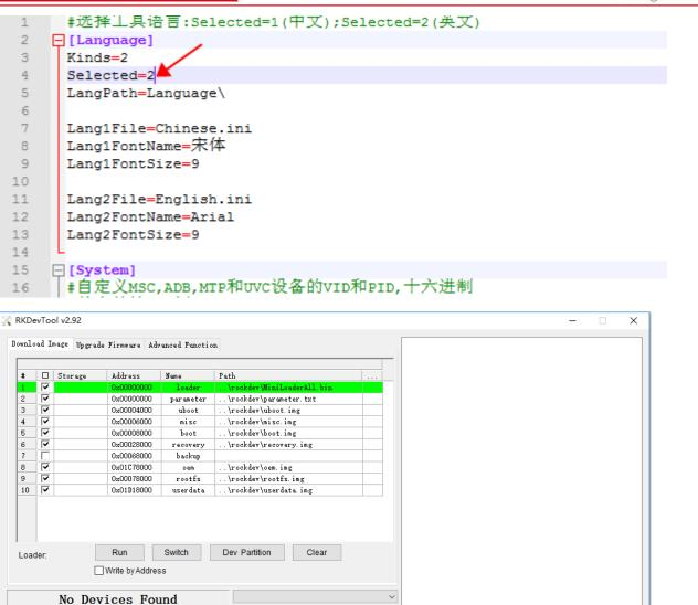
(3) Hold down the upgrade button (on the side of the board - as shown below), connect the PC via both USB burning cables, hold down the upgrade button for 5-10 seconds after power-on, until "Found One LOADER Device" (find a loading device) appears in the tool, see the picture below:
