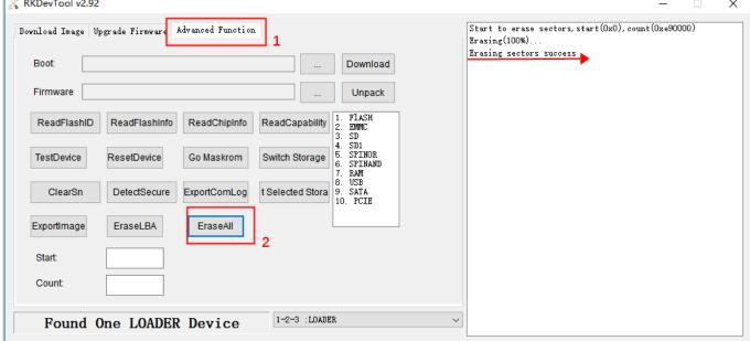
b. After the erasing is complete, power off and restart. The message "Found One MASKROM Device" is displayed, and then continue to perform Step 5 above to burn the system.
