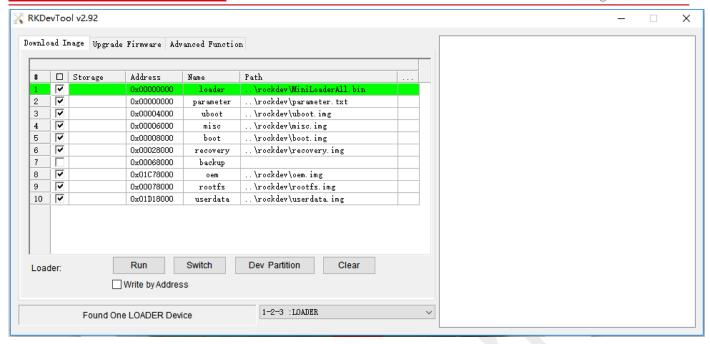
(4) Click "Upgrade Firmware" and click "Firmware" to load the update.img burning package. As follows:
