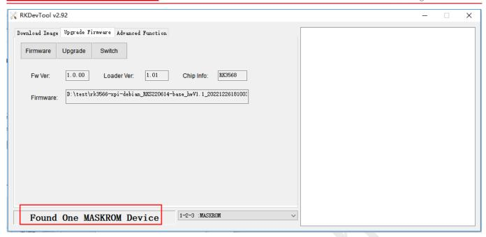
c. If the burning tool RKDevTool.exe can identify the LOADER/MASKROM Device, Rockusb Device can also be found in Device Manager on PC. If no, check whether the driver is installed properly or whether the steps are correct.
