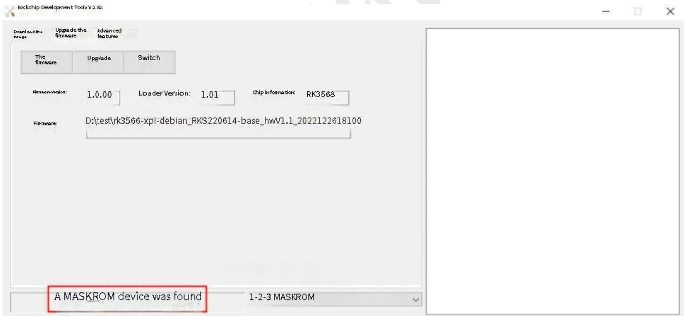
c. When the burning tool RKDevTool.exe can identify the LOADER/MASKROM device, the Rockusb Device can also be found in the "Device Manager" on the PC side. If not, please check whether the driver is installed normally or whether the steps are correct.
