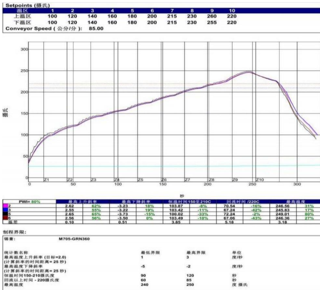
Reflow Temperature Profile
