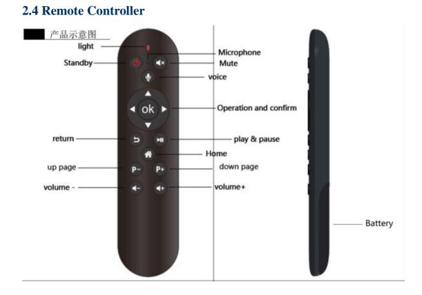
Note: Button Battery 2025 3V insert with correct polarity (+/-).
