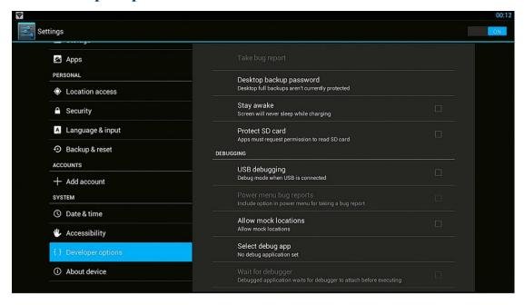
If user want to do some debugging on box by ADB, enable USB debugging, you will get ADB function by Ethernet or WiFi network.
